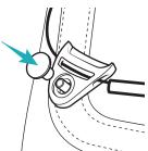
4 If satisfied with all placement, secure rivets using QuickFit™ Tool.
