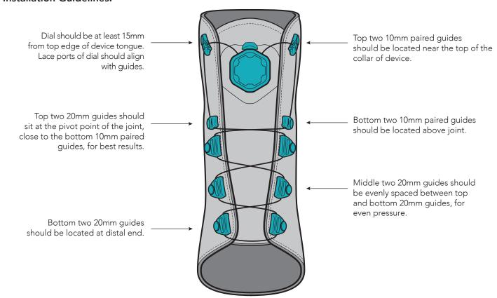
Determine guide and dial locations using installation guidelines. Punch holes using 1/8" punch option of QuickFit™ Tool.
