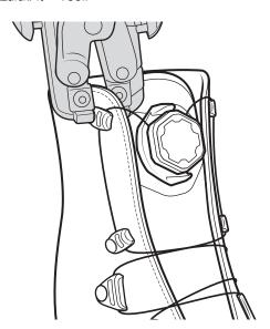
5 Rotate guides to correct lace alignment (see dashed line).
